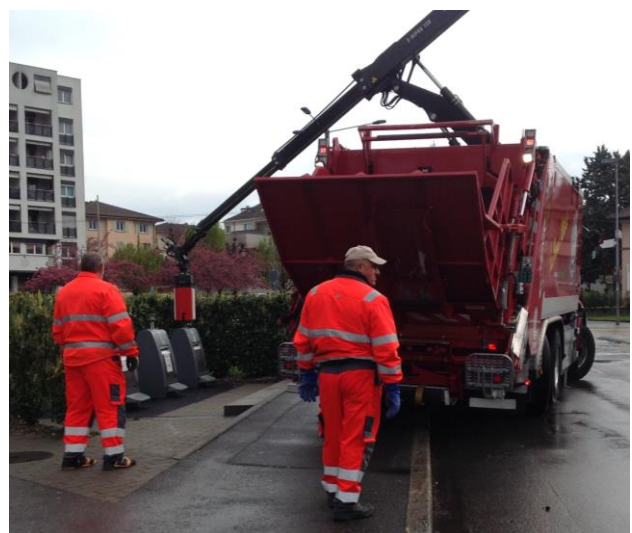
RENENS: THE CITY LIFTS BURIED CONTAINERS TO EMPTY THEM
